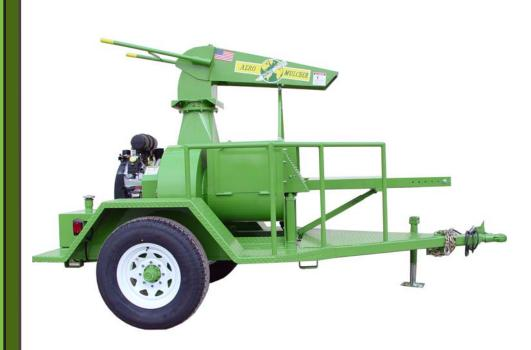
The **Bowie SG-50** is the intermediate workhorse of our manufactured Aero-Mulchers. This unit is powered by a Kohler EFI 38 HP Air Cooled Gas Engine to give years of trouble-free service. The discharge gun has a full 360° horizontal rotation and the fan is dynamically balanced. The six (6) blade 23" fan will generate an airflow of 4500 CFM at a velocity in excess of 120 MPH. The feed tray is fully adjustable with a detachable extension. This unit comes as either a skid or trailer mounted.
