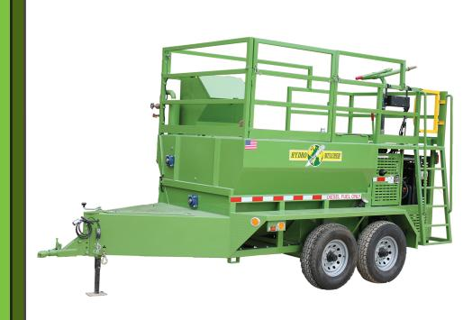
**Bowie's Victor 800** is one of our most popular Hydro-Mulchers. The low maintenance, ease of use and high productivity of the **Bowie Victor 800** Hydro-Mulcher® makes it a smart choice. With its many options, this piece of equipment makes it just right for your hydromulching needs. The trailer unit features a tandem 8000 lb. torflex axle, electric brakes on both axles, DOT approved LED running lights and an adjustable ball or pintle hitch.
